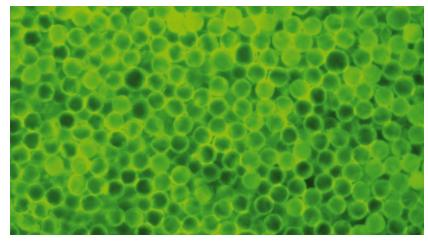
Fig. 4 Green Fluorescent Protein stained polystyrene microspheres with mean diameters of 10 microns showing a peak excitation wavelength of 480 nm, with a peak emission wavelength of 520 nm.
