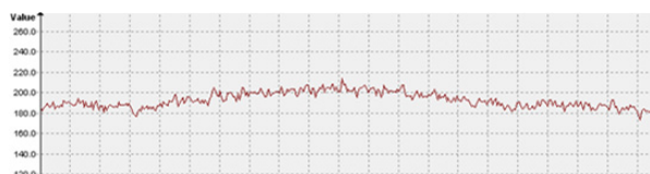
Pixel response before gain and offset correction
