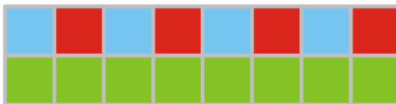
Bilinear sensor pixels with Green and alternating Red and Blue filters
