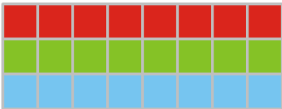
Trilinear sensor pixels with Red, Green, Blue filters per line
