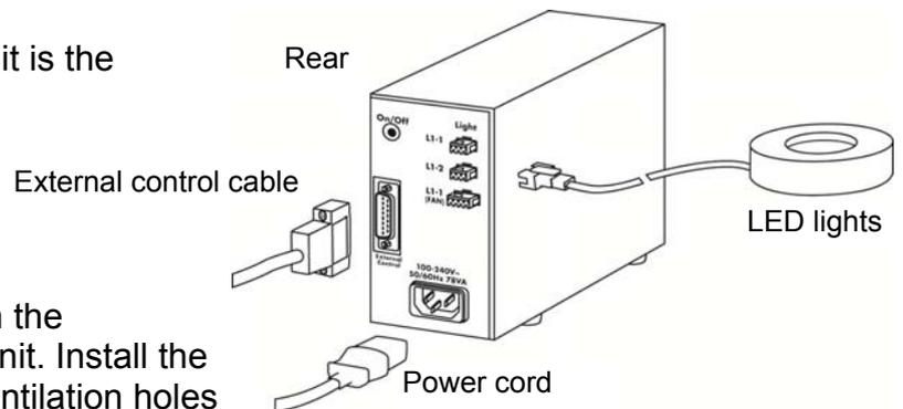
Note: There are fan ventilation holes on the PD2-5012/5024 Power Supply Unit. Install the Power Supply Unit so that the ventilation holes are not obstructed. (A clearance of 50 mm min. is recommended around the ventilation holes.)
