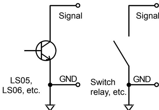
When using the PD2 in a noisy environment, we recommend that you isolate the signal and ground lines from the control unit with photo-couplers or photo-MOS relays. Any element that supplies around 10mA can be used to drive the circuit.
