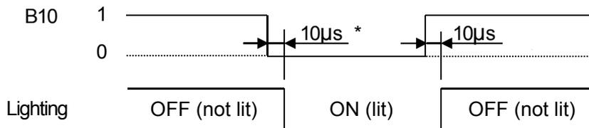
\*The delay is 10 µs when the light intensity is 100%. If the light intensity is less than 100%, there may be a delay of up to 30 µs.
