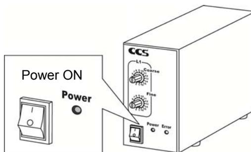
6. Use the intensity control knobs to set light intensity.
