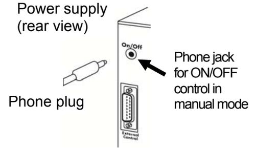
2. Insert the phone plug into the phone jack to send the ON/OFF control signal for manual control.
