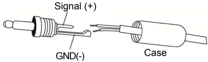
Contact your nearest CCS representative if you need to extend the control signal cable or operate in an extremely noisy environment. Cables should not be extended more than 3 m. Potentially harmful noise may be eliminated by installing a 0.01 to 0.1-  $\mu$  F capacitor between the signal and ground to ensure proper operation of this product. Phone plugs are not included with the power supply kit, but optional 3-m cables with plugs are available.
