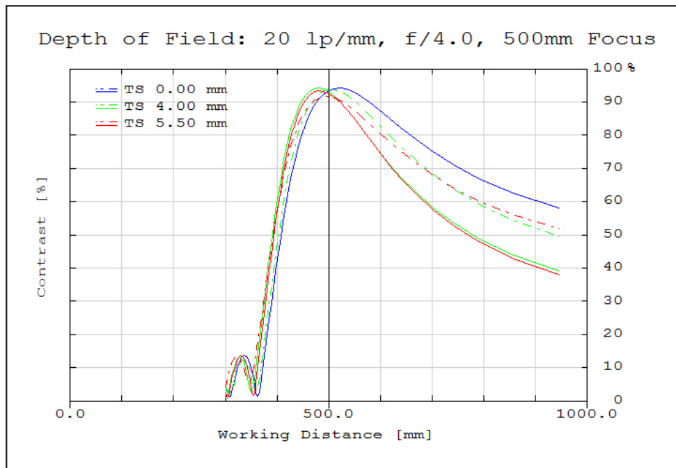
Figure 6: Polychromatic diffraction through-focus MTF at 20 linepairs/mm (image space). Contrast is plotted to two times the focus distance. Note object spatial frequency changes with working distance.
