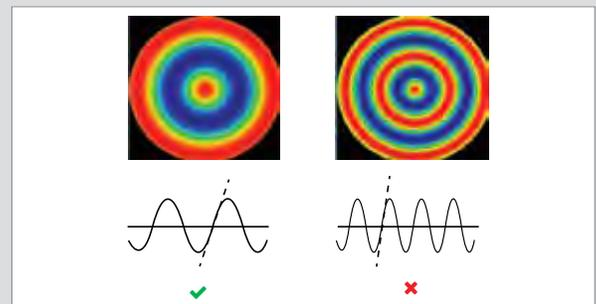
Figure 5: If a maximum slope specification is specified for the surface irregularity map, this creates a threshold to reduce the impact of higher spatial frequency content on the surface
