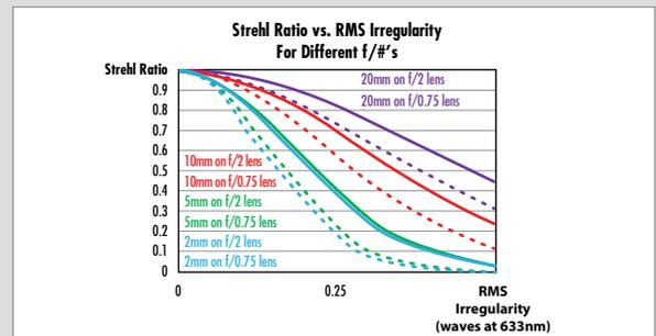
Figure 4: Comparing dotted lines to solid lines shows that a faster asphere (smaller  $f/\#$ ) has greater degradation compared to a slower asphere (larger  $f/\#$ ) over a given cosine period
