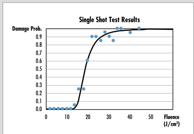
Figure 1: Sample data from a single shot test
