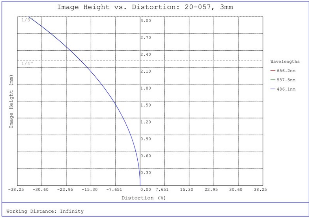
#20-057, 3mm FL f/5.6, IR-Cut Blue Series M12 Lens, Distortion Plot
