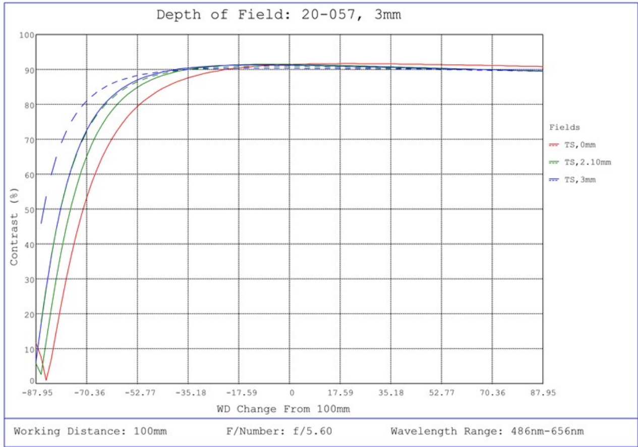
#20-057, 3mm FL f/5.6, IR-Cut Blue Series M12 Lens, Depth of Field Plot, 100mm Working Distance, f5.6
