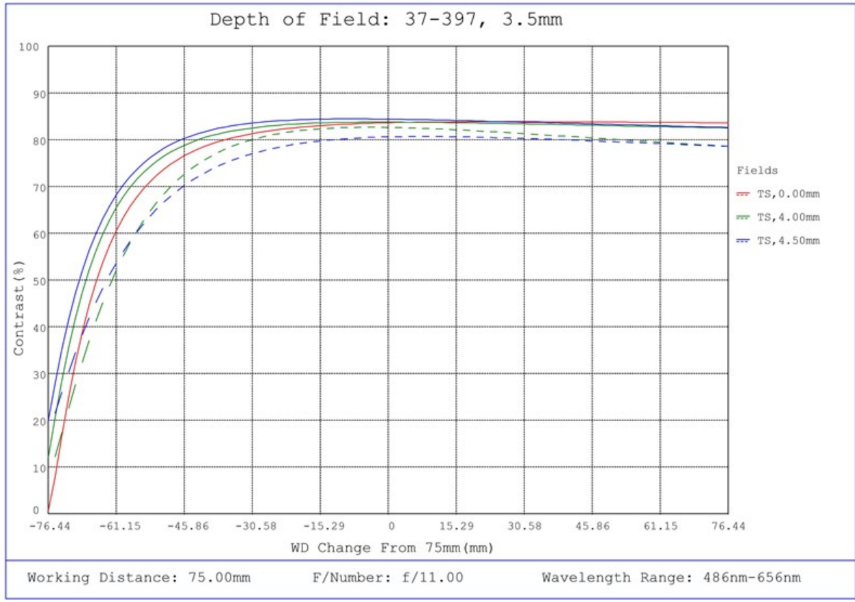
#37-397, 3.5mm, f/11 Cr Series Fixed Focal Length Lens, Depth of Field Plot, 75mm Working Distance, f11
