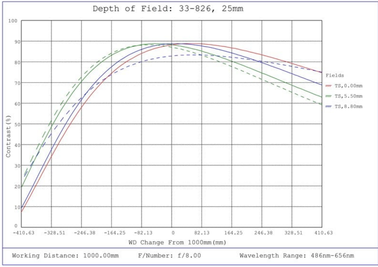
#33-826, 25mm f/8.0, HPI Series Fixed Focal Length Lens, Depth of Field Plot, 1000mm Working Distance, f8
