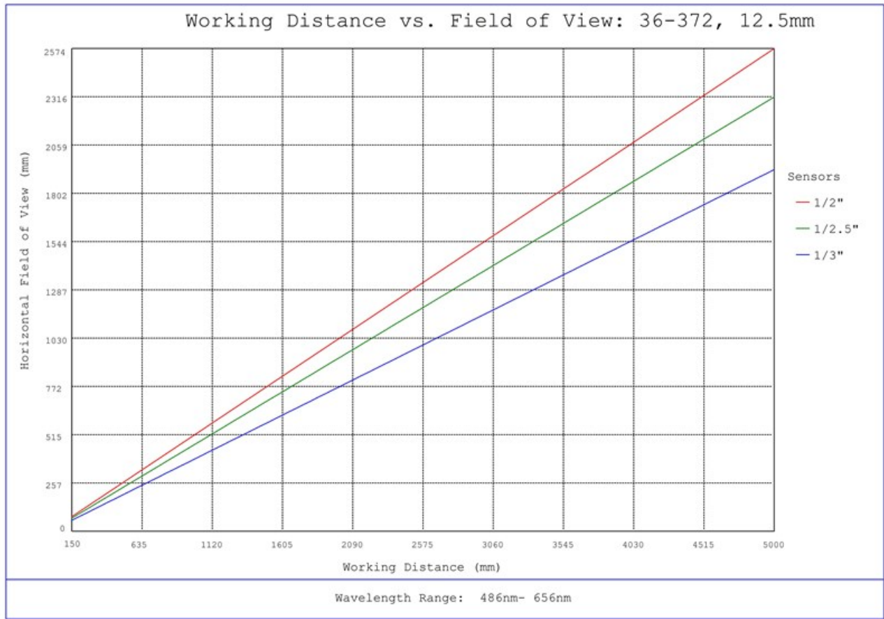
#36-372, 12.5mm FL f/2.5, Rugged Blue Series M12 Lens, Working Distance versus Field of View Plot
