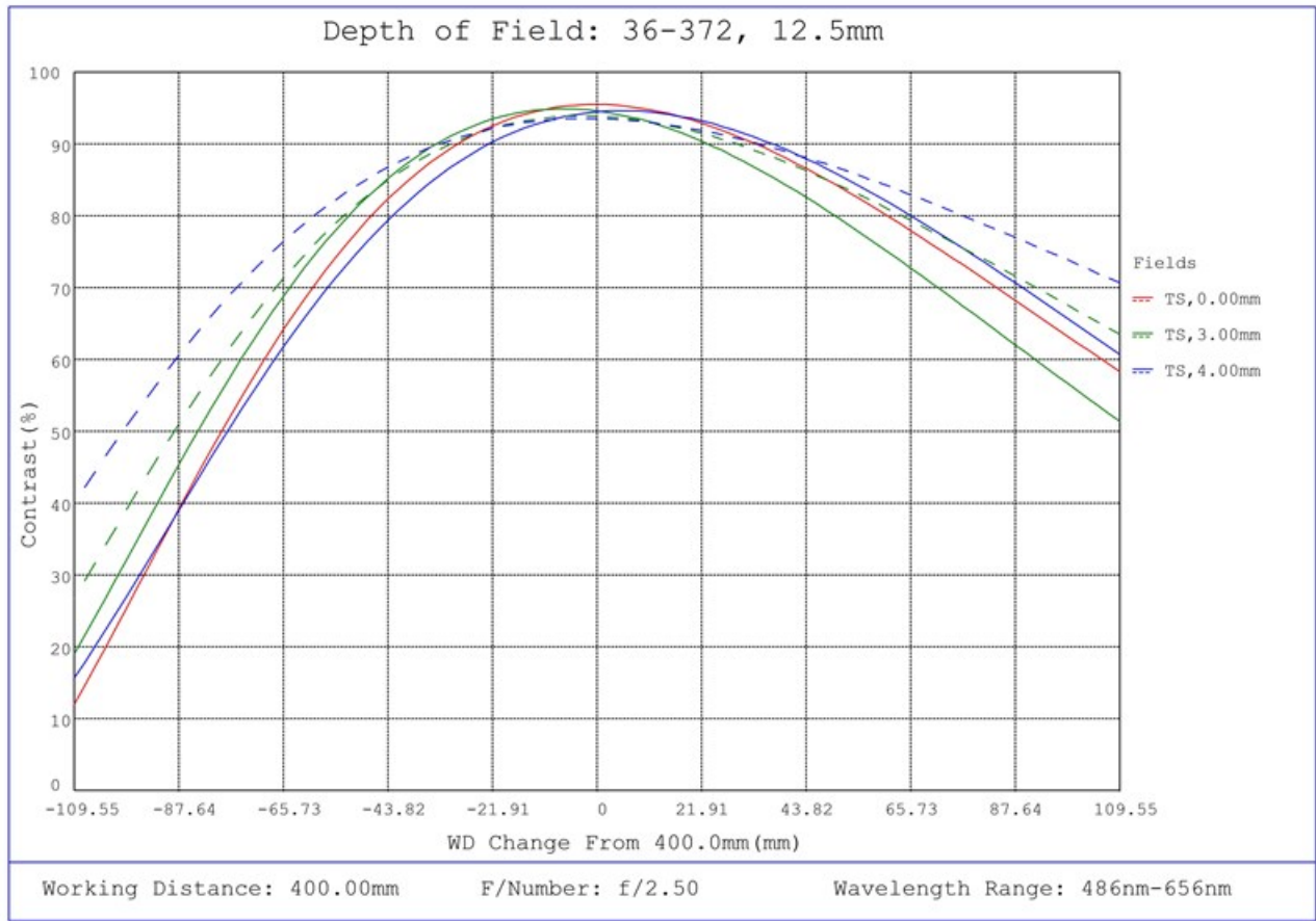
#36-372, 12.5mm FL f/2.5, Rugged Blue Series M12 Lens, Depth of Field Plot, 400mm Working Distance, f2.5
