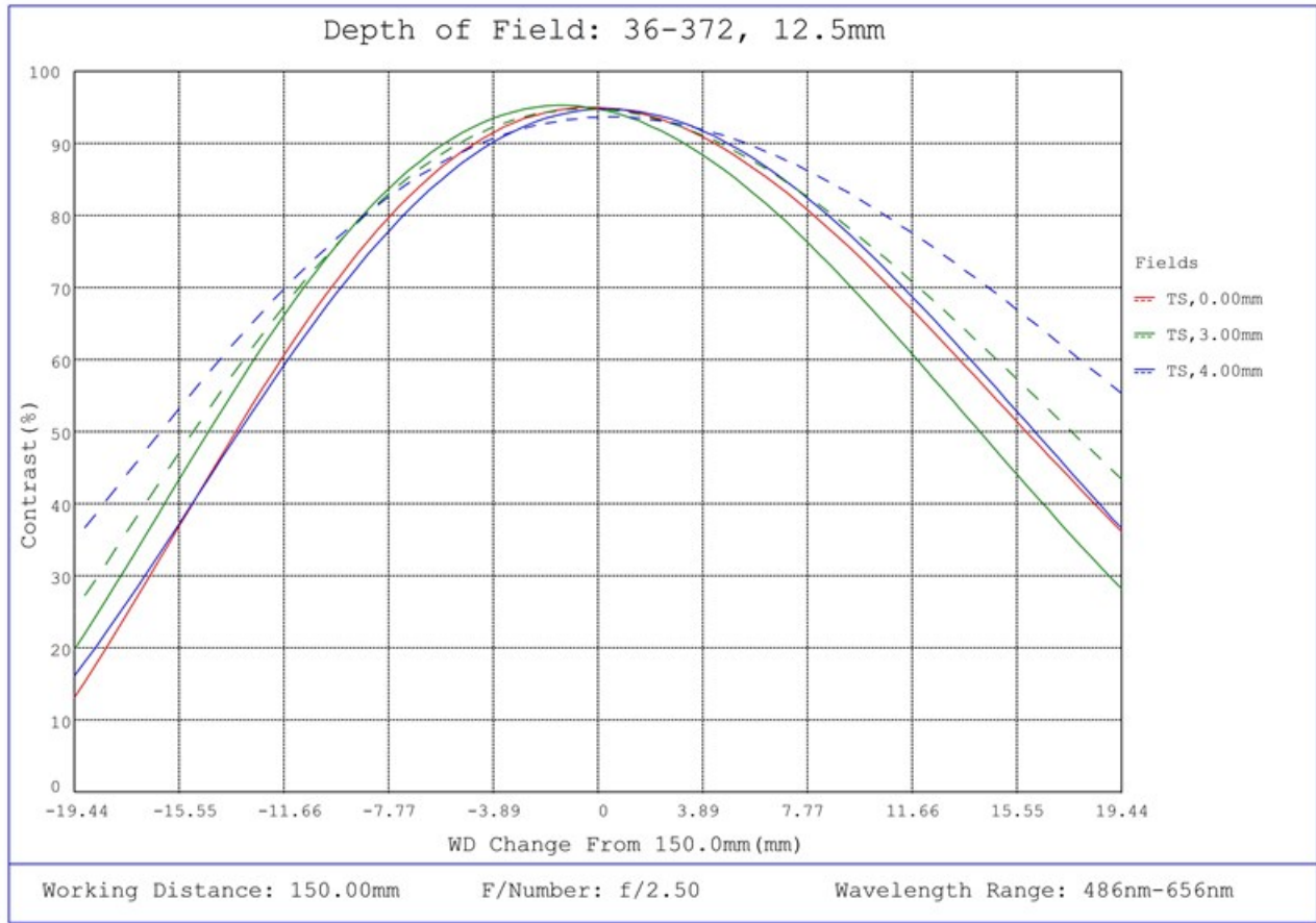
#36-372, 12.5mm FL f/2.5, Rugged Blue Series M12 Lens, Depth of Field Plot, 150mm Working Distance, f2.5
