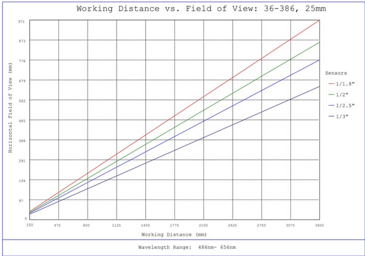
#36-386, 25mm FL f/5.6, Rugged Blue Series M12 Lens, Working Distance versus Field of View Plot
