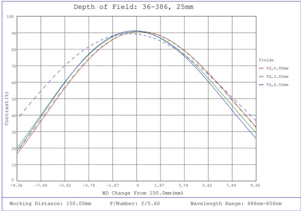
#36-386, 25mm FL f/5.6, Rugged Blue Series M12 Lens, Depth of Field Plot, 150mm Working Distance, f5.6
