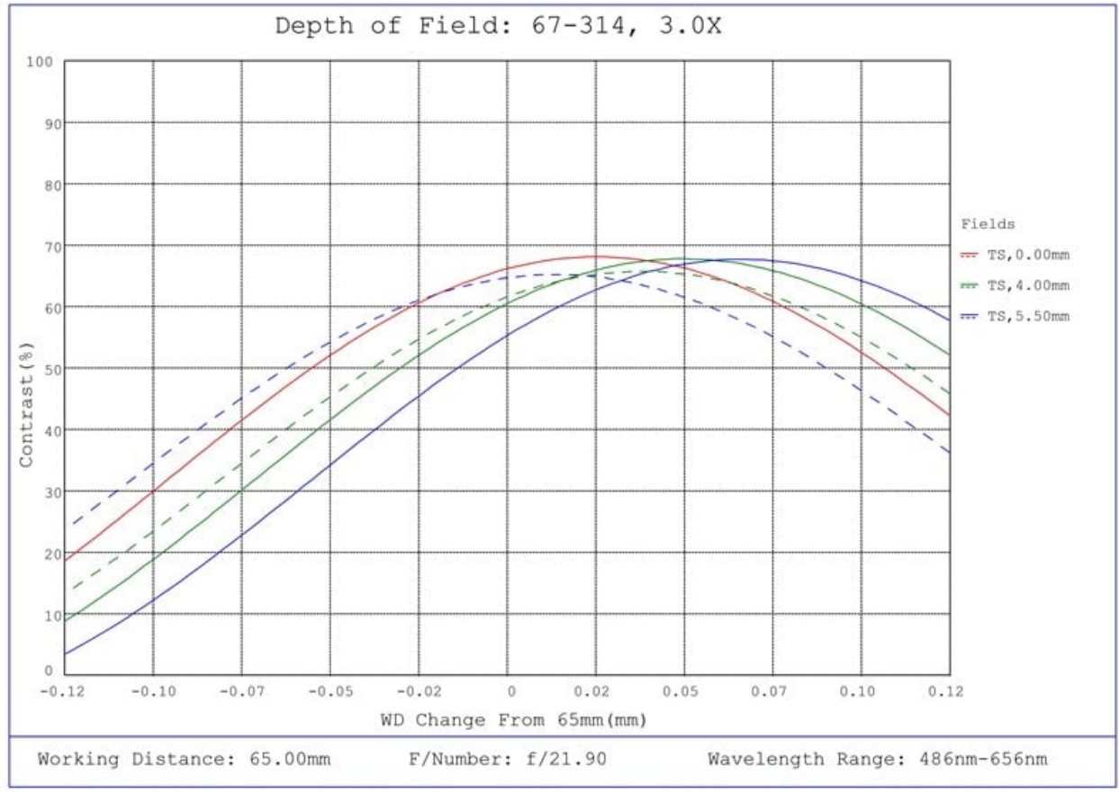
#67-314, 3X, 65mm WD, In-Line CompactTL™ Telecentric Lens, Depth of Field Plot, 65mm Working Distance, f21.9
