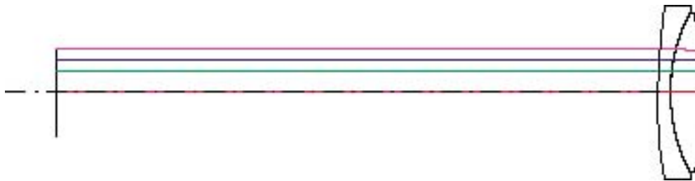
Figure B Telecentric lens drawing showing chief rays for each object point. Note that the chief rays are parallel to the optical axis.
